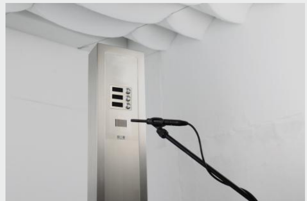
Pict. 3: Acoustic measurement of an intercom in our laboratory
