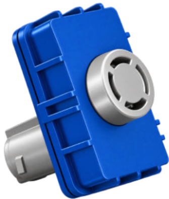
Fig. 1.: vicMIC A2B(O) external microphone (colours shown for illustrative purposes only; can be customised to customer specifications)
